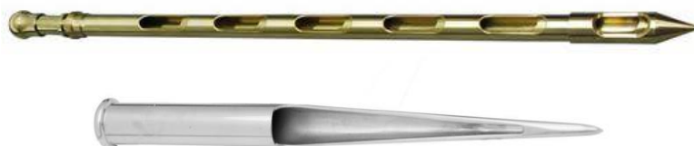
Figure 1: Example of a double tube grain probe (top) and bag trier (bottom; Gibson Company).
